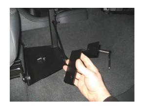
Install "Z" support bracket to base assembly using ¼ x ¾" carriage bolt and serrated nut.
